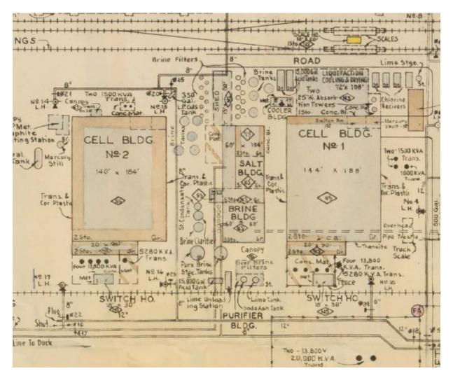
Leaks and spills of caustic solutions containing mercury, sodium hydroxide, sodium chloride brine, and bleach contaminated the sediments and ground water surrounding the cell buildings. Some liquid mercury was removed from the process equipment and from spaces beneath and between the building slabs after the cell buildings were demolished, and a soil cover was placed over the footprint of the buildings. A photograph taken during contaminated soil sampling/removal appears on the following page.
