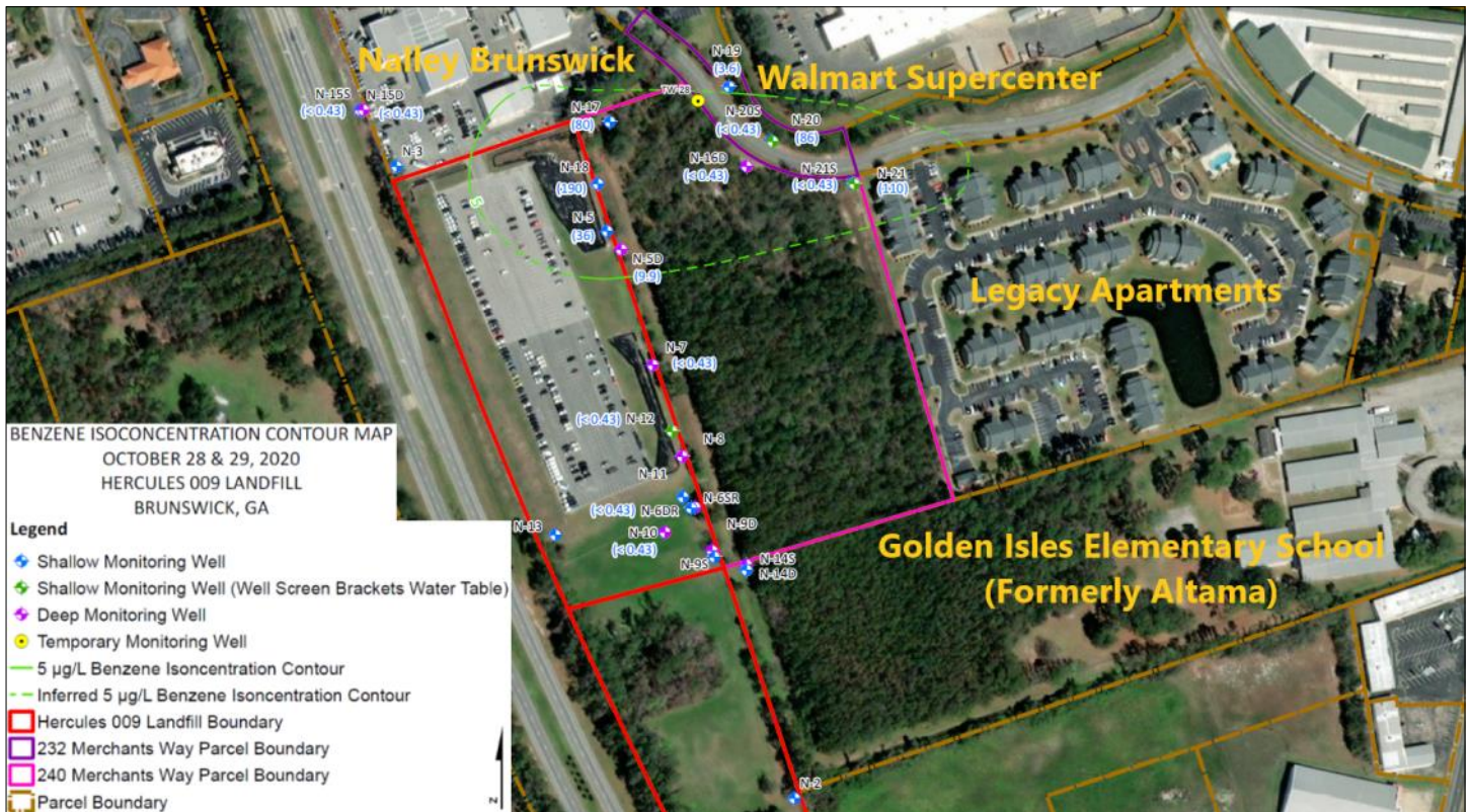
Approximate benzene ground water contamination based on new ground water monitoring data (does not include field screening results). Note the extent of the bright green line off-site. Ref: October 2021 Groundwater Assessment Report.
